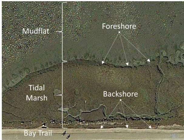
Figure 1.1. Aerial view of portion of Bothin Marsh showing relative positions of mudflat bayward of the marsh, foreshore between the marsh and mudflat, and backshore between the marsh and uplands, formed here by the Bay Trail.
