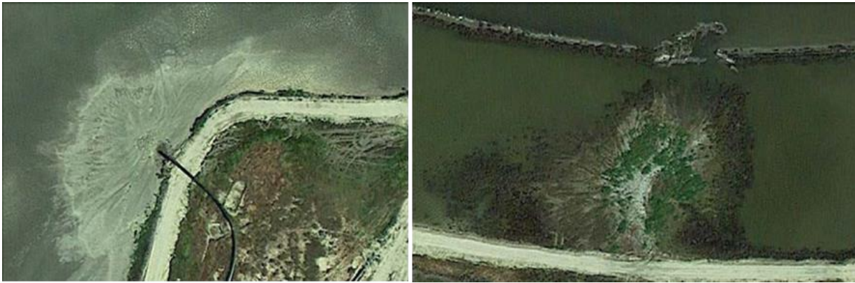
Figure 1.29. Montezuma Wetlands tidal marsh restoration project (Suisun Marsh) unintentionally created dredged sediment fans during filling of subsided diked baylands. Fans became vegetated with salt marsh vegetation prior to tidal restoration. April 2013 (Google Earth imagery).
